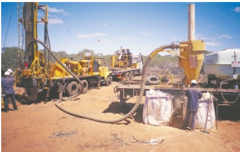
Drilling for bulk samples at Coburn, September 2002
